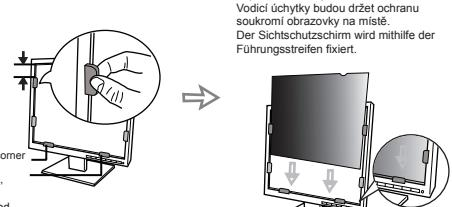
Place tab onto the bezel, 5-7cm from the corner of the screen.
