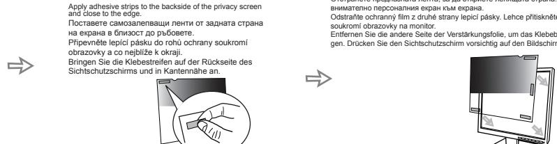
Remove the other side of the backing paper to reveal the adhesive. Gently press the privacy screen onto the screen.
