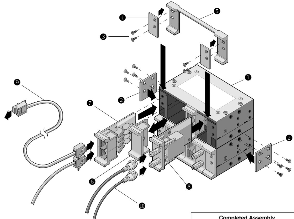
Figure 2. Side-by-Side Mounting
